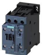
power contactor, AC-3 17 A, 7.5 kW / 400 V 1 NO + 1 NC, AC (50-60 Hz) DC operation 200-280 V AC/DC 3-pole, Size S0, screw terminal
