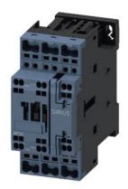
power contactor, AC-3e/AC-3, 17 A, 7.5 kW / 400 V, 3-pole, 208 V AC, 50/60 Hz, auxiliary contacts: 1 NO + 1 NC, spring-loaded terminal, size: S0
