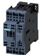
power contactor, AC-3e/AC-3, 17 A, 7.5 kW / 400 V, 3-pole, 230 V DC, auxiliary contacts: 1 NO + 1 NC, spring-loaded terminal, size: S0
