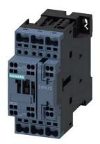
power contactor, AC-3e/AC-3, 17 A, 7.5 kW / 400 V, 3-pole, 24 V DC, with plugged-in diode combination, auxiliary contacts: 1 NO + 1 NC, spring-loaded terminal
