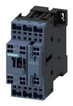
power contactor, AC-3e/AC-3, 17 A, 7.5 kW / 400 V, 3-pole, 21-28 V AC/DC, 50/60 Hz, with integrated varistor, auxiliary contacts: 1 NO + 1 NC, spring-loaded terminal, size: S0
