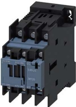
Traction contactor, AC-3 17 A, 7.5 kW / 400 V 1 NO + 1 NC with electronic drive 24 V DC, 0.7-1.25\* US, with integrated varistor, 3-pole, Size S0, ring cable lug connection
