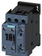
power contactor, AC-3e/AC-3, 25 A, 11 kW / 400 V, 1 NO + 1 NC, 24 V AC, 50 / 60 Hz, 3-pole, screw terminal
