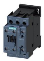
power contactor, AC-3e/AC-3, 25 A, 11 kW / 400 V, 3-pole, 100 V AC, 50 Hz / 100-110 V, 60 Hz, auxiliary contacts: 1 NO + 1 NC, screw terminal
