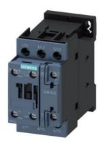
power contactor, AC-3e/AC-3, 25 A, 11 kW / 400 V, 3-pole, 230 V AC, 50 Hz, auxiliary contacts: 1 NO + 1 NC, screw terminal, upright mounting position
