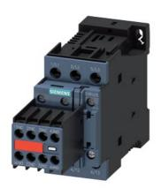
power contactor, AC-3e/AC-3, 25 A, 11 kW / 400 V, 3-pole, 24 V DC, with plugged-in varistor, auxiliary contacts: 2 NO + 2 NC, screw terminal, captive auxiliary switch
