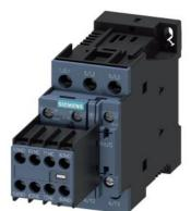
power contactor, AC-3e/AC-3, 25 A, 11 kW / 400 V, 3-pole, 24 V DC, with plugged-in diode combination, auxiliary contacts: 3 NO + 3 NC, screw terminal, with 3RH2911-1XA22-0MA0
