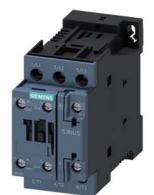
power contactor, AC-3e/AC-3, 25 A, 11 kW / 400 V, 3-pole, 21-28 V AC/DC, 50/60 Hz, with integrated varistor, auxiliary contacts: 1 NO + 1 NC, screw terminal
