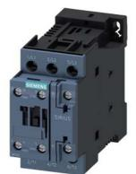
power contactor, AC-3e/AC-3, 25 A, 11 kW / 400 V, 3-pole, 95-130 V AC/DC, 50/60 Hz, with integrated varistor, auxiliary contacts: 1 NO + 1 NC, screw terminal
