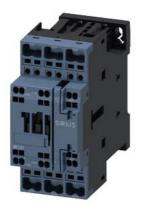
power contactor, AC-3e/AC-3, 25 A, 11 kW / 400 V, 1 NO + 1 NC, 110 V AC, 50 Hz / 120 V, 60 Hz, 3-pole, spring-loaded terminal
