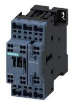
power contactor, AC-3e/AC-3, 25 A, 11 kW / 400 V, 3-pole, 24 V DC, auxiliary contacts: 1 NO + 1 NC, spring-loaded terminal, size: S0, upright mounting position
