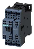
power contactor, AC-3e/AC-3, 25 A, 11 kW / 400 V, 3-pole, 12 V DC, 0.7-1.25\* Us, with plugged-in varistor, auxiliary contacts: 1 NO + 1 NC, spring-loaded terminal, size: S0, suitable for PLC outputs, not expandable with auxiliary switch
