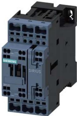
traction contactor, AC-3e/AC-3, 25 A, 11 kW / 400 V, 3-pole, 110 V DC, 0.7-1.25\* Us, electronic drive, with integrated varistor, auxiliary contacts: 1 NO + 1 NC, spring-loaded terminal
