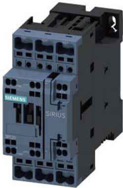
Traction contactor, AC-3 25 A, 11 kW / 400 V 1 NO + 1 NC with electronic drive 125 V DC, 0.7-1.25\* US, with integrated varistor, 3-pole, Size S0, Spring-type terminal
