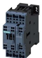
Traction contactor, AC-3 25 A, 11 kW / 400 V 1 NO + 1 NC with electronic drive 72 V DC, 0.7-1.25\* US, with integrated varistor, 3-pole, Size S0, Spring-type terminal
