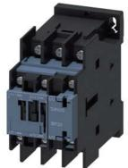
power contactor, AC-3e/AC-3, 25 A, 11 kW / 400 V, 3-pole, 100 V AC, 50 Hz / 100-110 V, 60 Hz, auxiliary contacts: 1 NO + 1 NC, ring cable lug connection, size: S0
