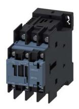
power contactor, AC-3e/AC-3, 25 A, 11 kW / 400 V, 3-pole, 24 V DC, 0.7-1.25\* Us, with plugged-in varistor, auxiliary contacts: 1 NO + 1 NC, ring cable lug connection, size: S0, suitable for PLC outputs, not expandable with auxiliary switch
