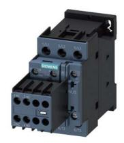
power contactor, AC-3e/AC-3, 32 A, 15 kW / 400 V, 3-pole, 400 V AC, 50 Hz, auxiliary contacts: 2 NO + 2 NC, screw terminal, size: S0, removable auxiliary switch
