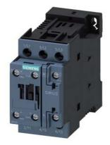
power contactor, AC-3e/AC-3, 32 A, 15 kW / 400 V, 3-pole, 125 V DC, auxiliary contacts: 1 NO + 1 NC, screw terminal
