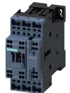
power contactor, AC-3e/AC-3, 32 A, 15 kW / 400 V, 3-pole, 125 V DC, auxiliary contacts: 1 NO + 1 NC, spring-loaded terminal, size: S0
