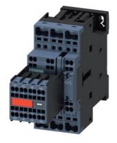
power contactor, AC-3e/AC-3, 32 A, 15 kW / 400 V, 3-pole, 110 V AC, 50 Hz / 120 V, 60 Hz, with plugged-in varistor, auxiliary contacts: 2 NO + 2 NC, spring-loaded terminal, size: S0, captive auxiliary switch
