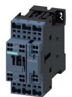
power contactor, AC-3e/AC-3, 32 A, 15 kW / 400 V, 3-pole, 95-130 V AC/DC, 50/60 Hz, with integrated varistor, auxiliary contacts: 1 NO + 1 NC, spring-loaded terminal
