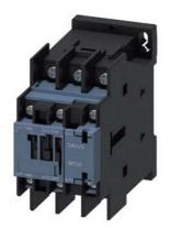
power contactor, AC-3e/AC-3, 32 A, 15 kW / 400 V, 3-pole, 100 V AC, 50 Hz / 100-110 V, 60 Hz, auxiliary contacts: 1 NO + 1 NC, ring cable lug connection, size: S0
