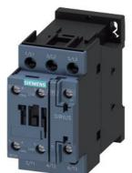
power contactor, AC-3e/AC-3, 38 A, 18.5 kW / 400 V, 1 NO + 1 NC, 24 V AC, 50 / 60 Hz, 3-pole, screw terminal
