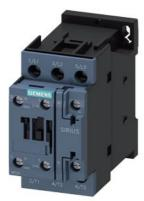
power contactor, AC-3e/AC-3, 38 A, 18.5 kW / 400 V, 3-pole, 110 V AC, 50/60 Hz, auxiliary contacts: 1 NO + 1 NC, screw terminal, India 40 A, Tu max. 50  $^{\circ}\text{C}$
