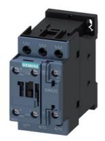
power contactor, AC-3e/AC-3, 38 A, 18.5 kW / 400 V, 3-pole, 48 V AC, 50/60 Hz, auxiliary contacts: 1 NO + 1 NC, screw terminal, size: S0
