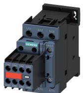
power contactor, AC-3e/AC-3, 38 A, 18.5 kW / 400 V, 3-pole, 110 V AC, 50 Hz / 120 V, 60 Hz, auxiliary contacts: 2 NO + 2 NC, screw terminal, captive auxiliary switch
