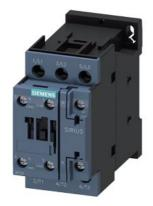
power contactor, AC-3e/AC-3, 38 A, 18.5 kW / 400 V, 1 NO + 1 NC, 220 V AC, 50 Hz / 240 V, 60 Hz, 3-pole, screw terminal
