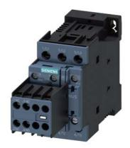
power contactor, AC-3e/AC-3, 38 A, 18.5 kW / 400 V, 3-pole, 110 V DC, auxiliary contacts: 2 NO + 2 NC, screw terminal, size: S0, removable auxiliary switch
