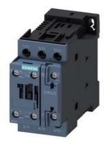
power contactor, AC-3e/AC-3, 38 A, 18.5 kW / 400 V, 3-pole, 200-280 V AC/DC, 50/60 Hz, with integrated varistor, auxiliary contacts: 1 NO + 1 NC, screw terminal
