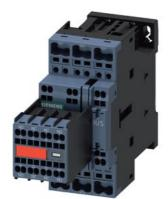
power contactor, AC-3e/AC-3, 38 A, 18.5 kW / 400 V, 3-pole, 110 V AC, 50 Hz / 120 V, 60 Hz, auxiliary contacts: 2 NO + 2 NC, spring-loaded terminal, size: S0, captive auxiliary switch
