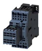
power contactor, AC-3e/AC-3, 38 A, 18.5 kW / 400 V, 3-pole, 24 V DC, auxiliary contacts: 2 NO + 2 NC, spring-loaded terminal, removable auxiliary switch
