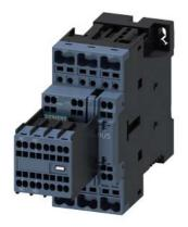
power contactor, AC-3e/AC-3, 38 A, 18.5 kW / 400 V, 3-pole, 110 V DC, auxiliary contacts: 2 NO + 2 NC, spring-loaded terminal, size: S0, removable auxiliary switch
