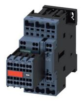
power contactor, AC-3e/AC-3, 38 A, 18.5 kW / 400 V, 3-pole, 110 V AC, 50 Hz / 120 V, 60 Hz, with plugged-in varistor, auxiliary contacts: 2 NO + 2 NC, spring-loaded terminal, size: S0, captive auxiliary switch
