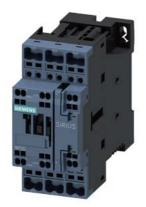
power contactor, AC-3e/AC-3, 38 A, 18.5 kW / 400 V, 3-pole, 21-28 V AC/DC, 50/60 Hz, with integrated varistor, auxiliary contacts: 1 NO + 1 NC, spring-loaded terminal, size: S0
