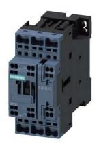
traction contactor, AC-3e/AC-3, 38 A, 18.5 kW / 400 V, 3-pole, 110 V DC, 0.7-1.25\* Us, electronic drive, with integrated varistor, auxiliary contacts: 1 NO + 1 NC, spring-loaded terminal
