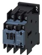
power contactor, AC-3e/AC-3, 38 A, 18.5 kW / 400 V, 3-pole, 110 V AC, 50 Hz / 120 V, 60 Hz, auxiliary contacts: 1 NO + 1 NC, ring cable lug connection, size: S0
