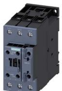
power contactor, AC-3e/AC-3, 41 A, 18.5 kW / 400 V, 3-pole, 110 V AC, 50 Hz / 120 V, 60 Hz, auxiliary contacts: 1 NO + 1 NC, screw terminal
