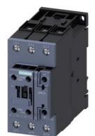
power contactor, AC-3e/AC-3, 41 A, 18.5 kW / 400 V, 1 NO + 1 NC, 24 V AC, 50 / 60 Hz, 3-pole, screw terminal
