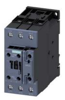
power contactor, AC-3e/AC-3, 41 A, 18.5 kW / 400 V, 3-pole, 208 V AC, 50/60 Hz, auxiliary contacts: 1 NO + 1 NC, screw terminal
