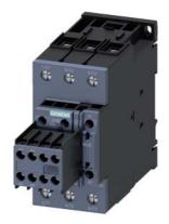
power contactor, AC-3e/AC-3, 41 A, 18.5 kW / 400 V, 3-pole, 230 V AC, 50 Hz, auxiliary contacts: 2 NO + 2 NC, screw terminal, removable auxiliary switch
