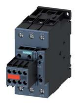
power contactor, AC-3e/AC-3, 41 A, 18.5 kW / 400 V, 3-pole, 110 V AC, 50 Hz / 120 V, 60 Hz, with plugged-in varistor, auxiliary contacts: 2 NO + 2 NC, screw terminal, size: S2, captive auxiliary switch
