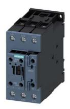
power contactor, AC-3e/AC-3, 41 A, 18.5 kW / 400 V, 3-pole, 20-33 V AC/DC, 50/60 Hz, with integrated varistor, auxiliary contacts: 1 NO + 1 NC, screw terminal, communication-capable
