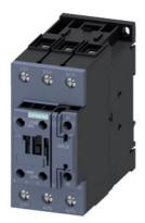
power contactor, AC-3 40 A, 18.5 kW / 400 V 1 NO + 1 NC, AC / DC 175-280 V, with varistor, 3-pole, Size S2, screw terminal
