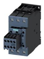
power contactor, AC-3e/AC-3, 41 A, 18.5 kW / 400 V, 3-pole, 175-280 V AC/DC, 50/60 Hz, with integrated varistor, auxiliary contacts: 2 NO + 2 NC, screw terminal, removable auxiliary switch
