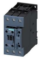
traction contactor, AC-3e/AC-3, 41 A, 18.5 kW / 400 V, 3-pole, 110 V DC, 0.7-1.25  $^{\star}$  Us, electronic drive, with integrated varistor, auxiliary contacts: 1 NO + 1 NC, screw terminal, size: S2
